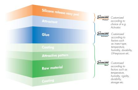
To apply the glue in exactly the right places does not of course solve all problems. The glue boards must also be designed to meet all requirements and needs. The glue boards must be easy to handle, the glue should not dry out. They must resist heat and UV-light, and be efficient. That's why the Silvalure® System Glue Board is built up like a sandwich, with three well-defined layers (see image) for maximum effect.
